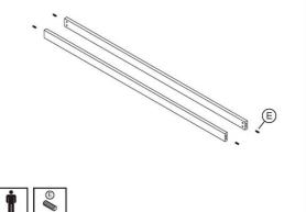
Fit the slat support (5)(6) to the back deck (1). Using Bolts ( C)(B) tighten with allen key (I). The back deck bundle is longer than the seat bundle. Identify the correct slat supports as shown below, and fit under the slats. Do not fully tighten any of the bolts yet!
