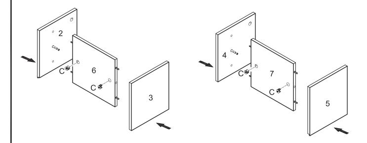
Insert cam locks (C) into shelves (6,7). Attach panels (2,3) to shelf (6) and panels (4,5) to shelf (7) using cam bolts and dowels as guides. Tighten cam locks (C) with a screwdriver to secure panels (2,3) to shelf (6) and panels (4,5) to shelf (7).
