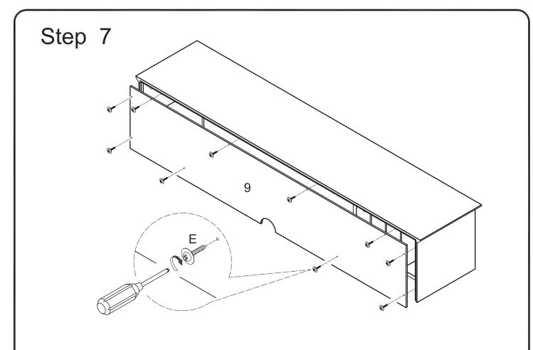
Attach back panel (9) to the hutch assembly using screws (E).
