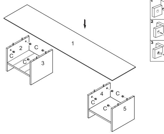
Insert cam locks (C) into panels (2,3,4,5). Attach hutch top (1) to the panel assemblies using cam bolts and dowels as guides. *Insure that the thin grooves across one end of hutch top (1) are above shelf (6).* Tighten cam locks (C) to secure hutch top (1) to the panel assemblies.
