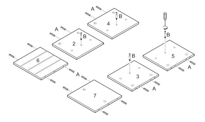
Insert dowels (A) into panels (2,3,4,5) and shelves (6,7). Screw cam bolts (B) into panels (2,3,4,5).
