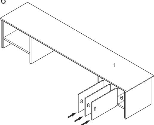
From the back of the hutch assembly, carefully slide divider panels (8) into place along the grooves of hutch top (1) and shelf (6).
