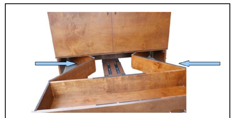
6) To fold back into cabinet, reverse steps 5 and 4. ENSURE THE SAFETY LATCH IS ON. Then fold in the bifold rails as shown above. Push in drawer pedalstal until flush with cabinet, then lock side latches.
