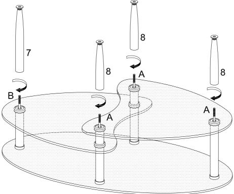
Screw leg (7) onto short rod (B). Screw legs (8) onto long rods (A). Ensure that legs (7,8) fit snuggly into the decorative rings placed in the previous step.
