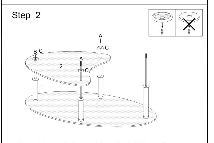
Slide glass (2) then decorative rings (C) onto short rod (B) and middle long rods (A).
