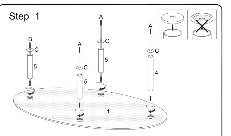
Carefully lay top glass (1) up-side-down on a soft surface. Screw short rod (B) into the left plate of top glass (1). Screw long rods (A) into the middle and right plates of top glass (1). Slide cylinders (5) onto short rod (B) and middle long rods (A). Slide cylinder (4) onto right long rod (A). Slide decorative rings (C) onto rods (A,B) and snap onto cylinders (4,5).
