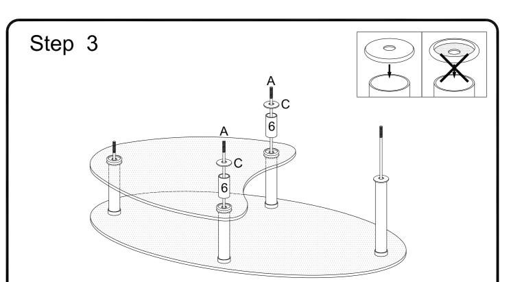
Slide cylinders (6) onto middle long rods (A). Ensure that cylinders (6) fit snuggly into the decorative rings placed in the previous step. Slide decorative rings (C) onto middle long rods (A) and snap onto cylinders (6).
