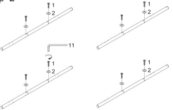
Secure the post sections from STEP 1 together using small bolts (1) with small washers (2). Tighten small bolts (1) with small wrench (11).
