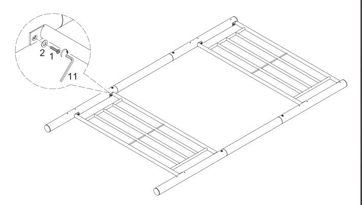
Secure guardrails (P) to the assembled posts from STEP 2 using small bolts (1) with small washers (2). Tighten small bolts (1) with small wrench (11). Repeat this step for both sets of guardrails and posts.
