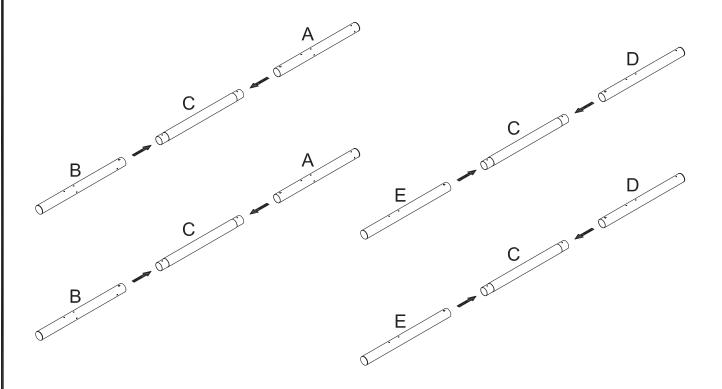
Slide post sections (A,B) and post sections (D,E) onto post sections (C). Ensure that the holes of all post sections align as shown above.
