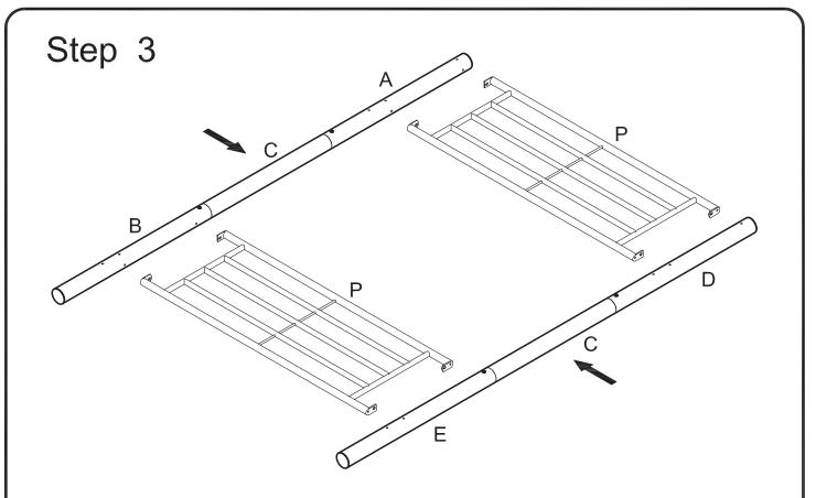
Place guardrails (P) between the assembled posts from STEP 2. Repeat this step for both sets of guardrails and posts.
