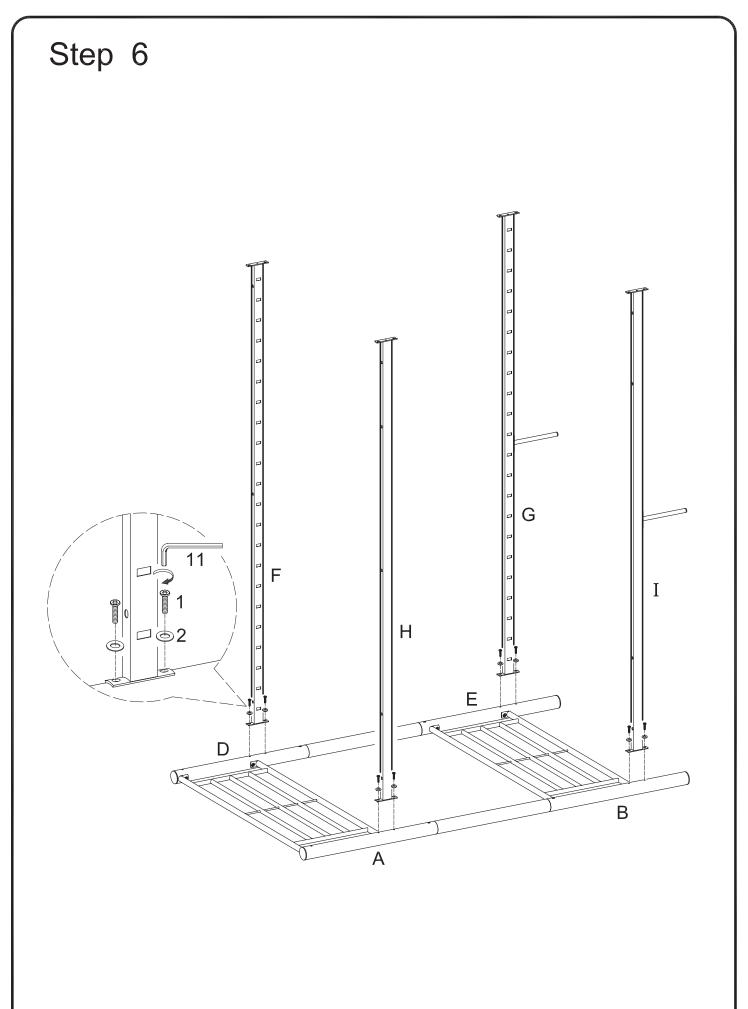
Attach crossbars (F,G,H,I) to corresponding post sections (D,E,A,B) as shown above using small bolts (1) with small washers (2). Tighten small bolts (1) with small wrench (11).
