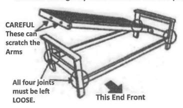
B. When you have the Back deck fitted lying flat, tighten all the Bolts. From the back, lift the Back Deck to upright as illustrated. Be careful not to scratch the Arms with the Plastic Runners when you lower the ends of the Back Deck. Your arm style may vary
