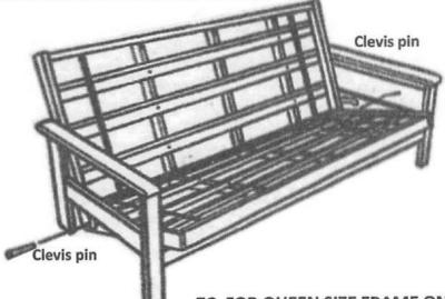
Fit the seat deck between the Arms and into the Back Deck as shown. Use the Clevis Pins to connect the two decks. Secure with a washer and Locking Pin.
